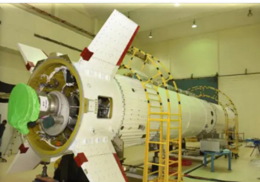
Test vehicle for characterisation of Crew Escape System ready at SDSC
